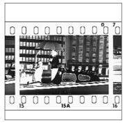
When dry, examine the negatives. The film edges (rebates) should be clear, with legible frame numbers along the bottom. A correctly exposed and processed negative should have a full range of tones, with some parts almost clear (like the rebates) and other parts so dense you can only just read print through them. Handle your negatives by the edges only.
