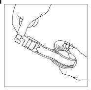
Add 5ml/l (1+200) of ILFOTOL wetting agent to the final rinse water, stir briefly, then lift the film spiral out of the tank. Pull the end of the film out of the spiral, and securely attach a wooden or plastic film clip to it (to get a tight grip you may have to double over the end of the film).
