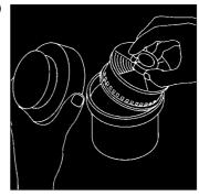
Continue step 7 until you reach the end of the film, then cut this away from the cassette spool. Give a few extra turns to wind the film all the way on. Finally, put the spiral into the developing tank with its plastic sealing ring (if needed), and screw on the tank lid. The film is now sealed inside a light-tight container, so you can switch on the room lights.
