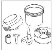
Set out the film and equipment in a logical order, so that you will be able to find them in the dark. You need only the equipment to get the film out of the cassette and into the light-tight developing tank.
