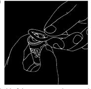
Take hold of the cassette and your end cap remover and turn out the light. Lever the cap off the cassette, and slide the film spool part way out. Find the film's shaped leader, slot this through the light-trap opening, then slide the spool back. This saves having 1.4m/4ft 8in of loose film falling on the floor.
