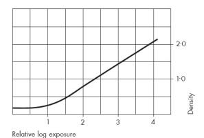
HP5 Plus film developed in ILFORD ILFOTEC HC (1+31) stock for  $6\frac{1}{2}$  minutes at  $20^{\circ}\text{C}/68^{\circ}\text{F}$  with intermittent agitation. This curve is also representative of roll film and sheet film formats.
