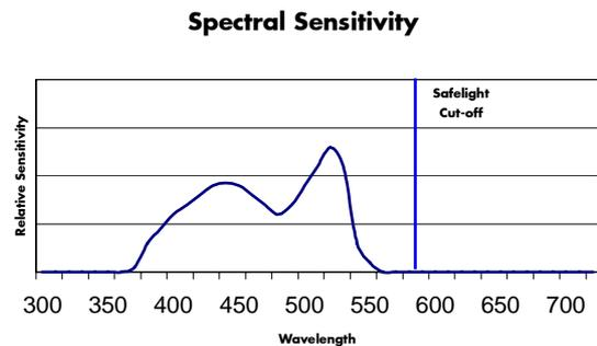
Use an appropriate safelight with a cut-off of no lower than 580nm – either a dark brown or red type.
