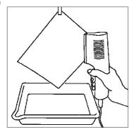
After the wash, drain the print and use a squeegee or sponge to remove any excess water. Attach a wooden or plastic clip to one corner, and hang the print over a drip tray to dry. Drying can be speeded up by using a hairdryer on a low setting, kept moving and about 30cm/1ft away from the print. MULTIGRADE prints dry naturally in a warm room in under 30 minutes.
