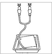
Wash the print for 2 minutes in a good flow of water ideally at about 20°C/68°F but cold water above 5°C/41°F will give adequate washing. Empty the wash tray a few times to ensure a complete change of wash water, or use rubber tubing to syphon water from the bottom of the tray.
