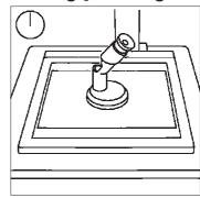
With the lens at full aperture, turn on the enlarger. Place an easel loaded with a spare piece of paper on the baseboard. Move the enlarger head to frame and focus the image. You can use a special 'focus finder' placed in the centre of the image to focus on the negative grain for the sharpest possible image.
