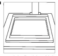
Switch the room light off and, by safelighting, position the easel under the enlarger to frame the print as you want it. Take out a new sheet of MULTIGRADE paper, and place this on the easel. Using the timer, give the paper the correct exposure worked out by examining the test print.
