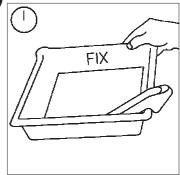
Slide the paper into the dish of fixer, and rock the dish to get a good flow of chemicals over the surface of the print. Fixing takes only 30 seconds in fresh solution. It does not matter if this time is exceeded slightly, but prints should not be left in the fixer for minutes on end. If not washing a print straight away, store it in a dish of clean water.
